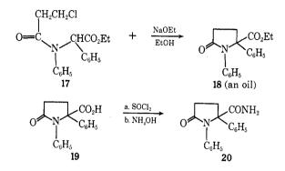
diphenylpyrrolidine-2-carboxylate (18) was prepared under conditions similar to those used for the preparation of 2. Compound 18 (an oil) was readily hydrolyzed to the crystalline acid 19, which was then converted to the amide 20. Similarly, the cyclization of diethyl N-(3-bromopropionyl)anilinomalonate to 2,2-dicarbethoxy-1-phenyl-5-oxopyrrolidine is reported.<sup>1,2</sup>
